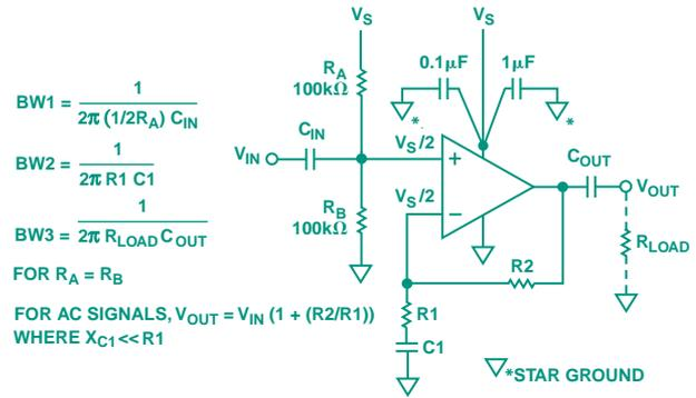
Figure 1. A potentially unstable single-supply op amp circuit.
