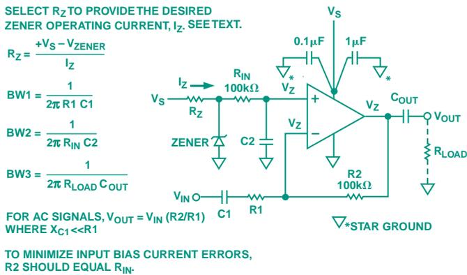
Figure 5. An inverting single-supply amplifier using Zener-diode biasing.
