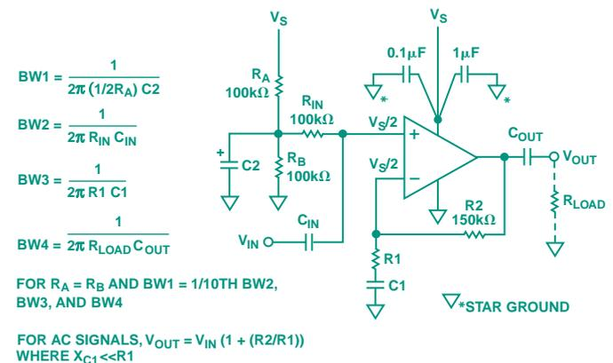
Figure 2. A decoupled single-supply op amp biasing circuit.
